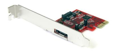
The PEXSAT31E1 2-Port PCI Express SATA/eSATA 6 Gbps (SATA 3.0) Controller Card adds one internal SATA 3.0 (6 Gbps) and one external eSATA 3.0 (6 Gbps) port, through a single PCIe slot.
