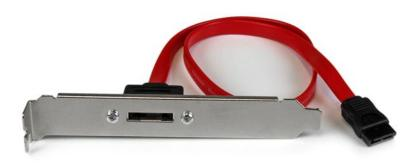
The ESATAPLT18IN 18-inch 1-port SATA to eSATA plate adapter adds external data support using an existing motherboard Serial ATA controller. Simply mount the plate to the rear panel of your computer case as an extension of the motherboard SATA data connector, in order to add a port for connecting external SATA storage devices (e.g. external eSATA hard drive).
