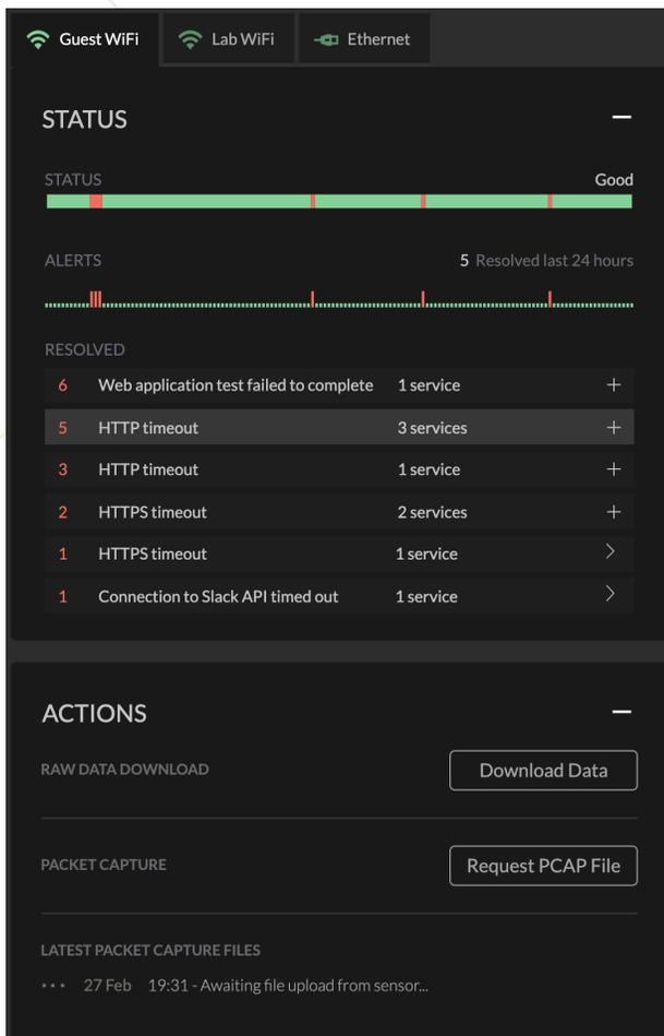
UXI sensors use dynamic packet captures that are uploaded to the cloud when issues are detected. The packet capture data is invaluable for troubleshooting issues in depth and arriving at root cause without having to visit the site. Reported data includes: connectivity, throughput, latency, jitter, packet loss, web server response time, web application transaction time and VoIP MoS.
