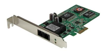
The PEX1000MMSC2 PCIe Gigabit Fiber Network Card lets you connect a desktop PC directly to a fiber optic network, by adding a multimode SC fiber port to your computer or server through an available PCI Express slot.
