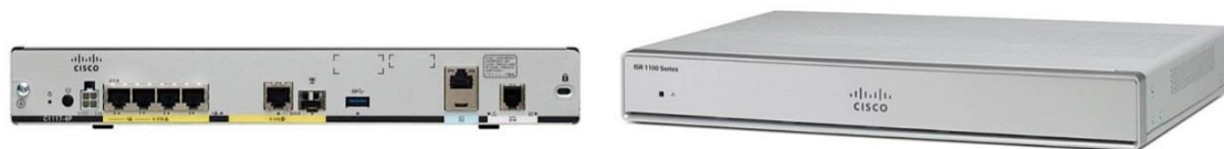
Figure 2. Cisco 1100-4P ISR, back and front views
