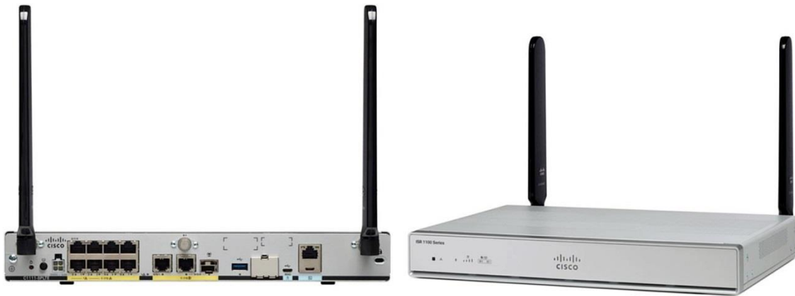
Figure 2. Cisco 1100-4P ISR, back and front views
