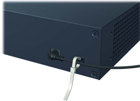
Figure 2-8. Using the cable tie on the HP 2530 8-port switches with external power supply
