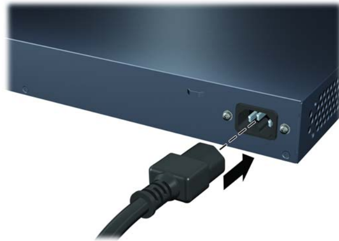
Figure 2-7. Connecting the power cord on the 2530-48G-PoE+ Switch
