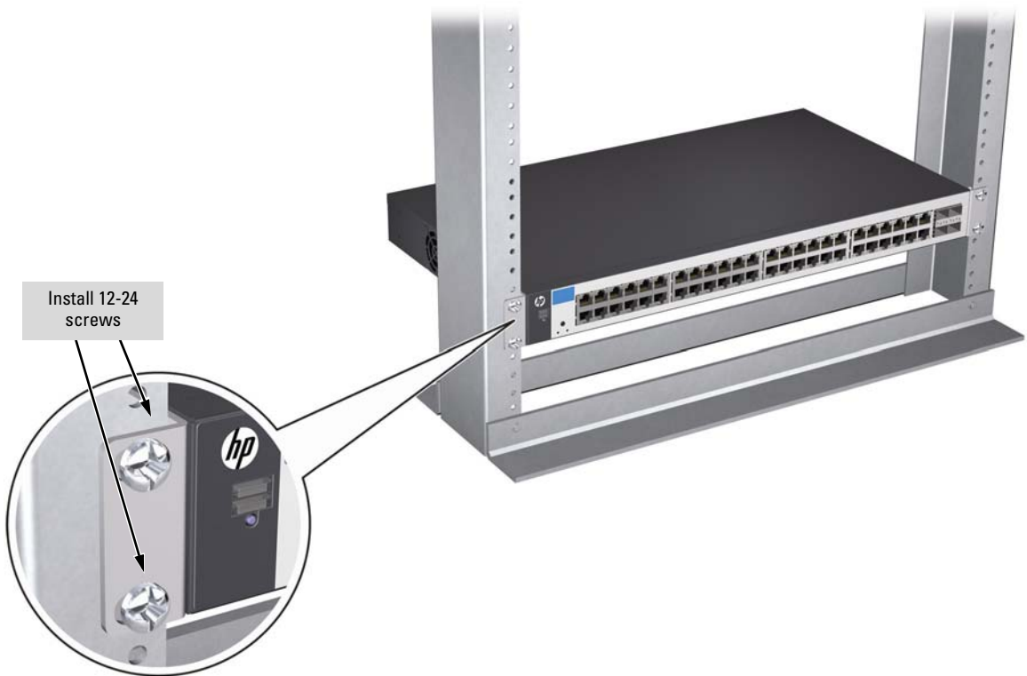
Figure 2-4. Mounting in a rack
