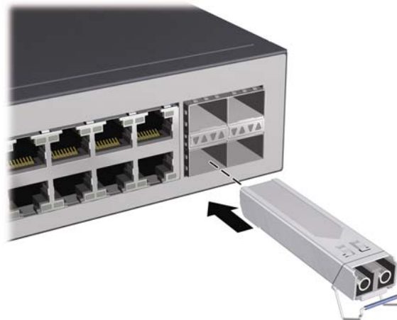
Figure 2-10. Installing an SFP
