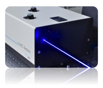
The GWU-UHG series is a user-friendly Harmonic generation module capable of second, third, and fourth harmonic generation for ultrafast oscillators with options for pulse selection.
