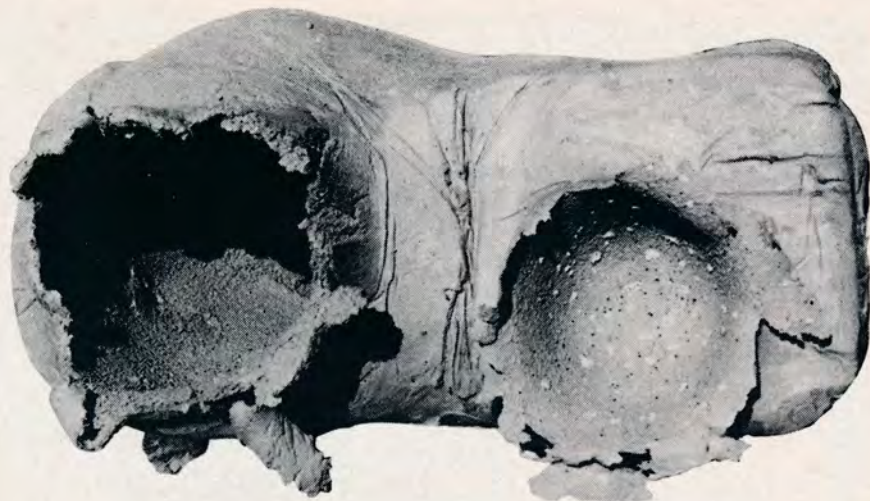
Comparative impacts on 6 x 6 clay block shows dramatic results. Left, 110-grain Super Vel .357 Magnum penetrated completely leaving a 5½" cavity. The impact of an 11-grain wax-plastic bullet, right, created a crater about 4-inches in diameter and 2½-inches deep. The bullet disintegrated on impact and shed all its energy. Wounds induced by such an impact would cause severe shock and could possibly be fatal. Further testing is needed.
