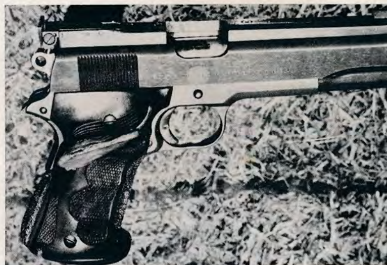
The rear sight as furnished by Elliason, plus a heavy rib. The rear sight is adjustable for both windage and elevation. The weight of the rib on the slide tends to dampen rise of the muzzle under the heavy .45 recoil.
