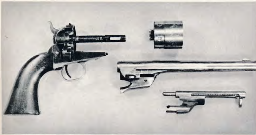
The major parts used in the C. B. Richards conversion of a Model 1860 Colt .44 Army caplock to shoot the .44 Colt metallic cartridge disassembled for viewing.
