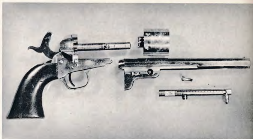
Major parts for the Richards-Mason method of converting a .36 caliber caplock Navy pistol to use a .38 caliber metallic cartridge are shown clearly above.
