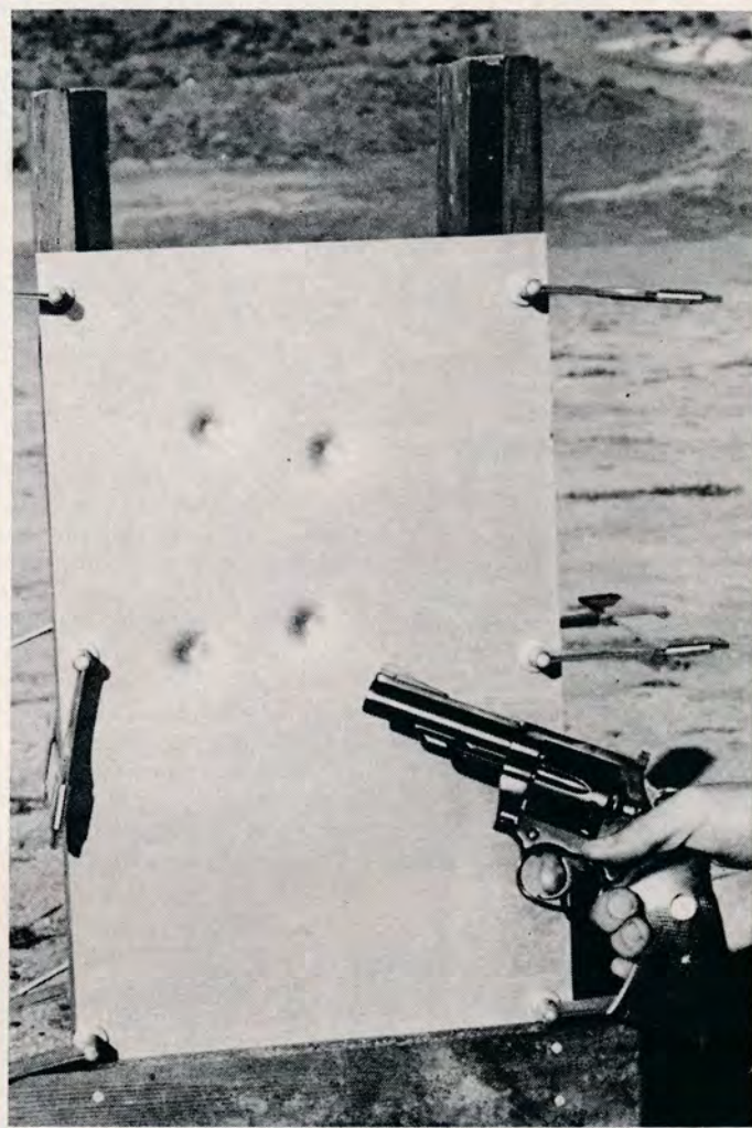
Impact of maximum anti-hijack loads caused only slight dimpling of sheet aluminum equivalent in strength to the lightest weight material used for jetliner skins. The gun is Colt's Mark III Trooper, .357, 4" barrel.
