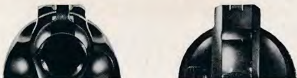
These two views of the partridge sight best show the correct sight picture from both the muzzle end and the shooter's view. System is best because it provides points of reference for precise aim.
