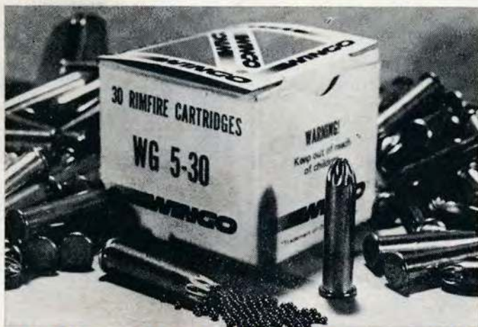
Special ammunition is used for the Wingo gun. The .20 caliber rimfire shotshell fits only in the special gun; no other ammunition will fit the chamber. Ammunition contains 119 #12 birdshot and spreads to a 20-inch pattern at 40 feet, compared to 125 pellets contained in the .22 long rifle shotshell. Gun is smooth-bored.
