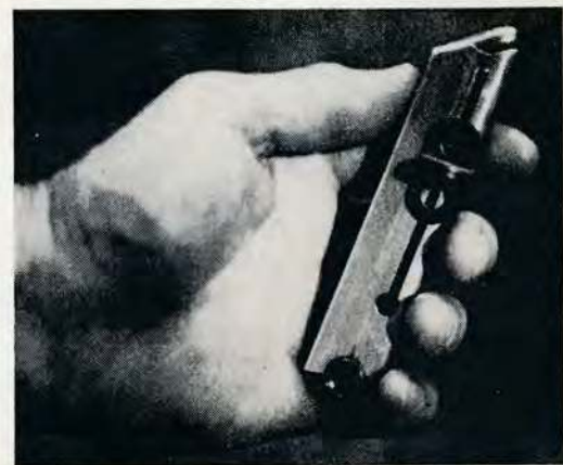
This is the tool supplied with the .380 as an aid in loading the magazine. It is merely stamped metal but it saves thumbs and fingers in an operation that would be a chore without it. A good design feature.
