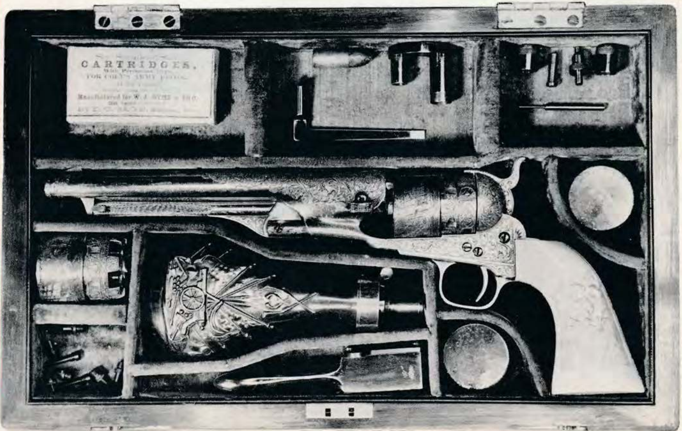
One of the finest cased pistols ever produced by Colt. Now in the Phillips collection, this handsome outfit was obtained by the author in Spain. Along with the regular percussion cylinder this Model 1860 Army pistol is also designed to use a conversion ring and accompanying Thuer front loading cartridge cylinder; necessary loading tools for the rare metallic tapered cartridges are also included in the case. Note label on the cartridge box.
