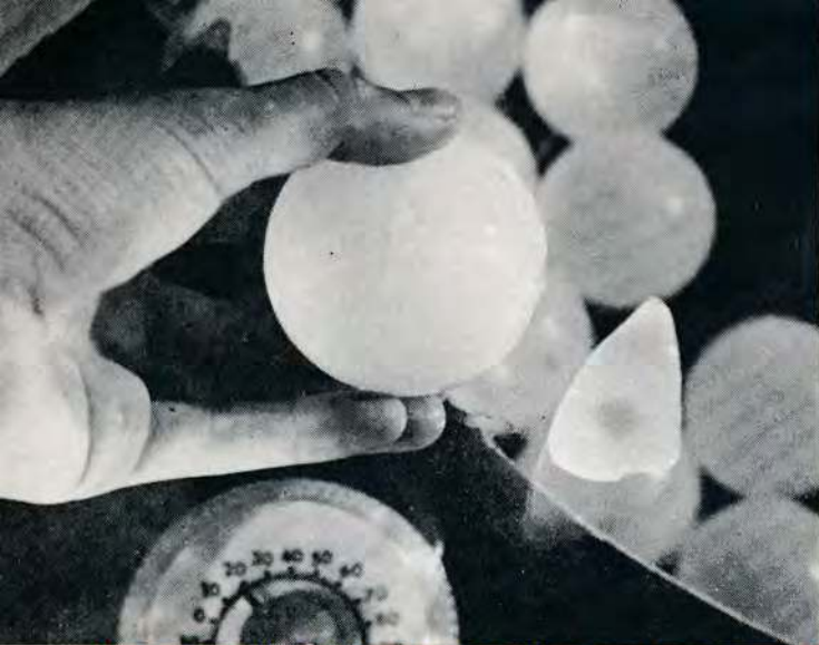
The unique Wingo target. Note the sectioned piece of one of the targets showing the 1/10th-inch thickness of the walls. The center of the mould is visible between the thumb and little finger of the hand holding the ball. Targets are stored in the freezer cabinet in the background until they are ready for launching.
