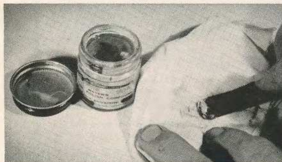
Polishing compound is put on cloth, and permitted to dry a bit before applying.
