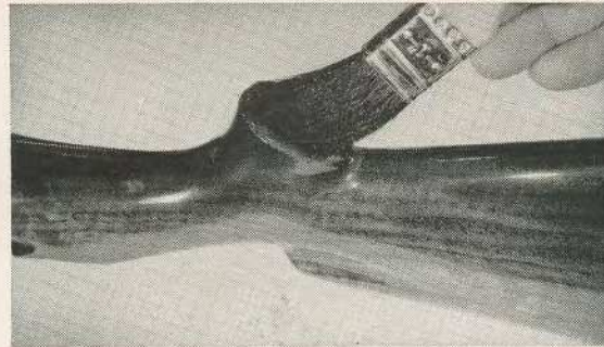
Surface under the grip cap also has open end grain, and it should be thoroughly protected.
