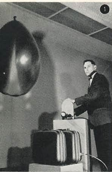
Ray gun fits in suitcase, yet one pulse of Laser light of 1/2000th second duration cut through steel plate to burst balloon 10' beyond. It may also burst balloons of bombast and threats frequently launched from behind Iron Curtain.
