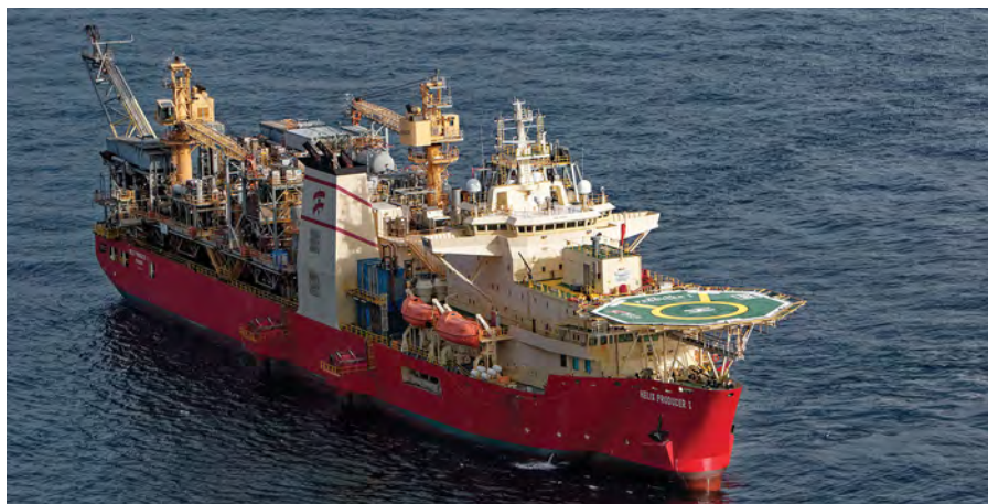
One of the few floating production facilities operating in the Gulf of Mexico, the Helix Producer I receives oil and gas production from subsea wells at Talos' Phoenix complex in the Green Canyon area. Image: Talos Energy.
