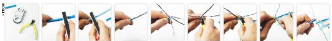
Prepare your tools. Use the cable stripper tool and cut the outer sheath. Cut the outer foil. Remove the foil. Separate all pairs and the drain wire. Cut and remove the foil of the first pair. Cut and remove the foil of the second pair. Cut and remove the foil of the third pair. Cut and remove the foil of the fourth pair.
