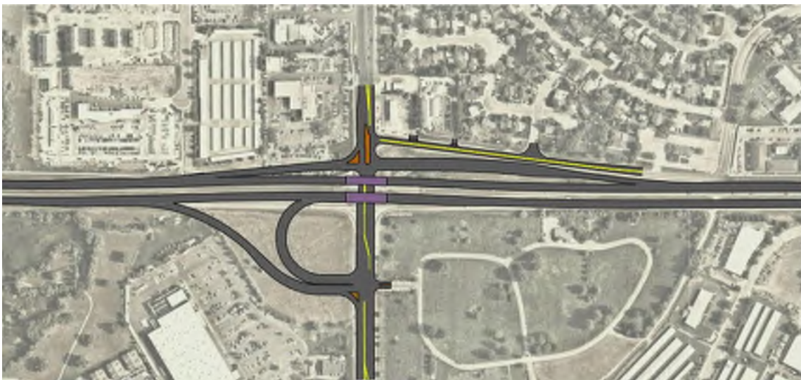
Figure 2.7 – Tight Diamond with D-Loop
