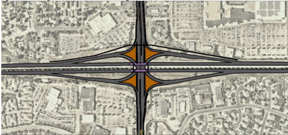
Figure 4.3 – Single Point Urban Interchange (SPUI)
