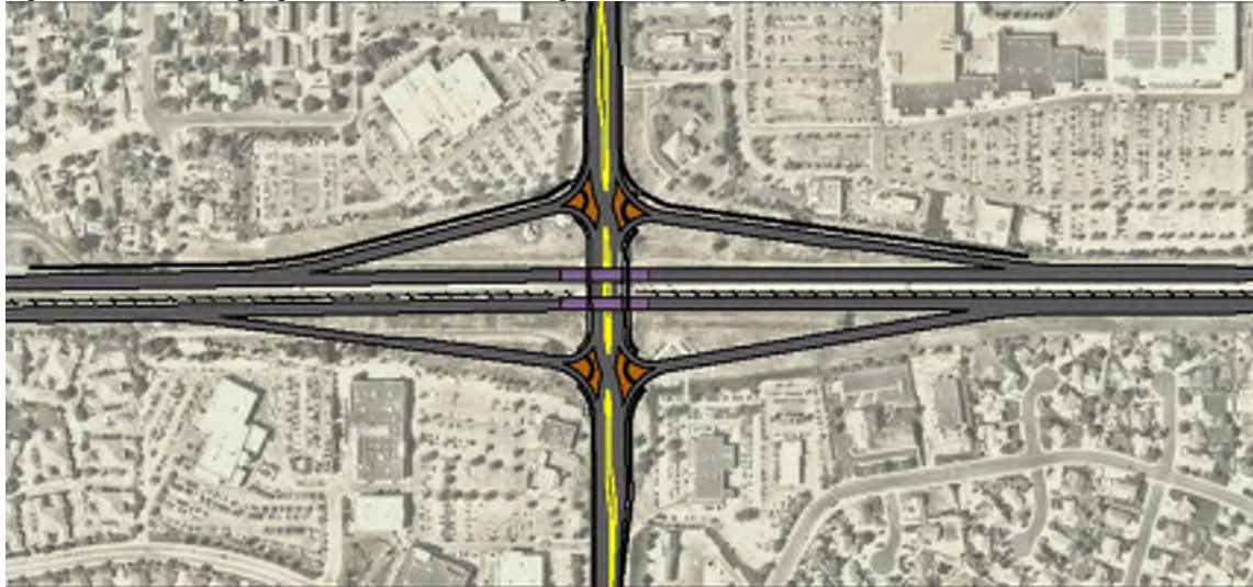
Figure 4.2 – Diverging Diamond Interchange (DDI)
