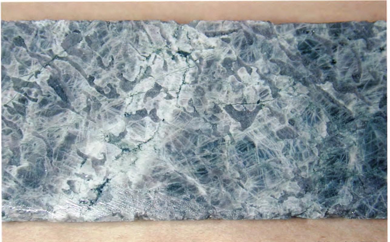
Plate 18 Graphic intergrowths of quartz and feldspar in pegmatite (hole 2002 @ 51.8 m).
