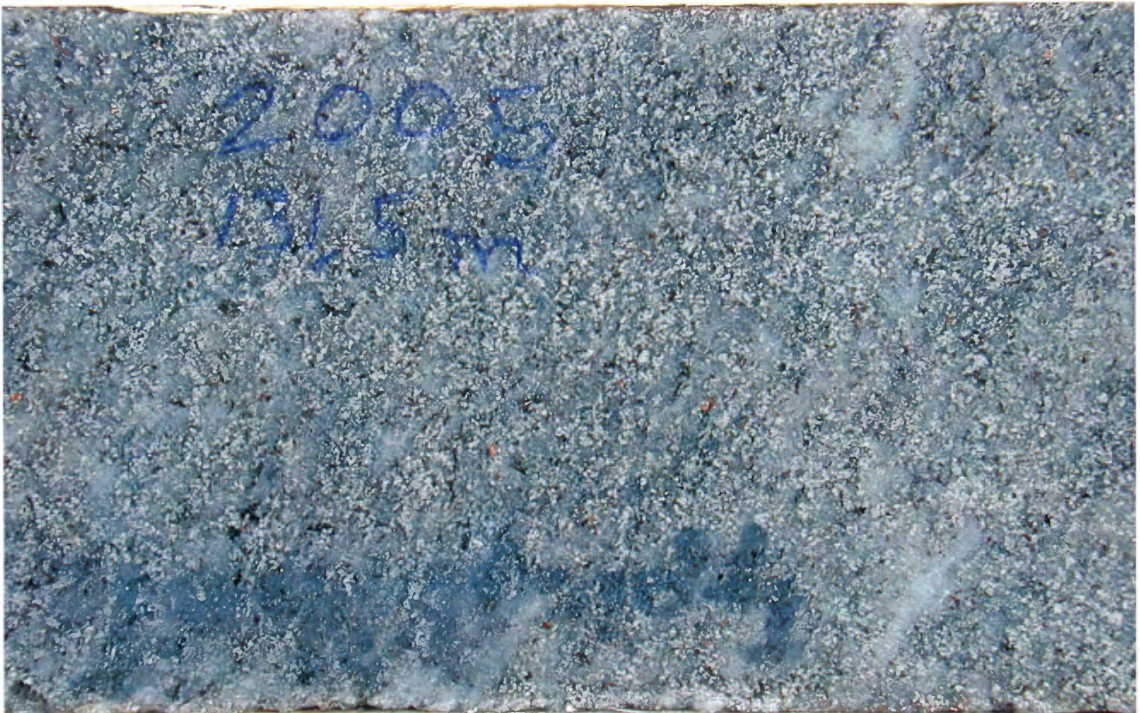
Plate 14 Weakly foliated, nonmagnetic, fine grained, intergranular bluish norite (hole 2005 @ 131.5 m).
