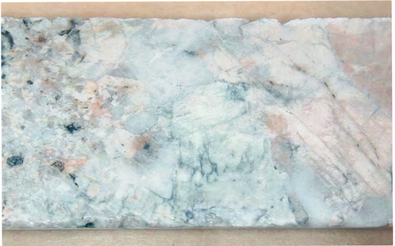
Plate 15 Potassium feldspar-rich margin of a tonalitic pegmatite (hole 2002 @ 163 m).
