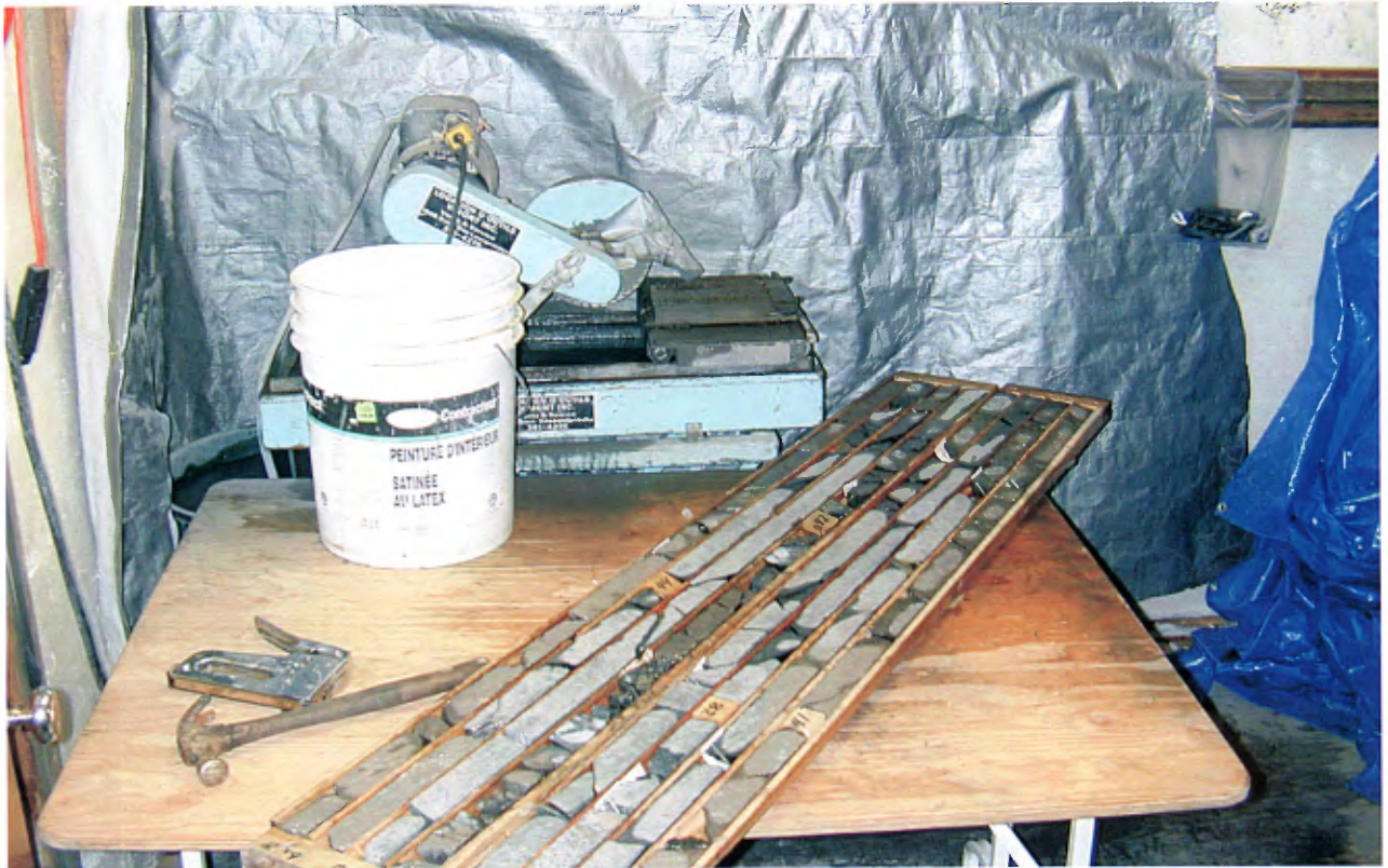
Plate 5 Sampled diamond saw cut BQ diamond drill core. Sample intervals marked by white assay tags.
