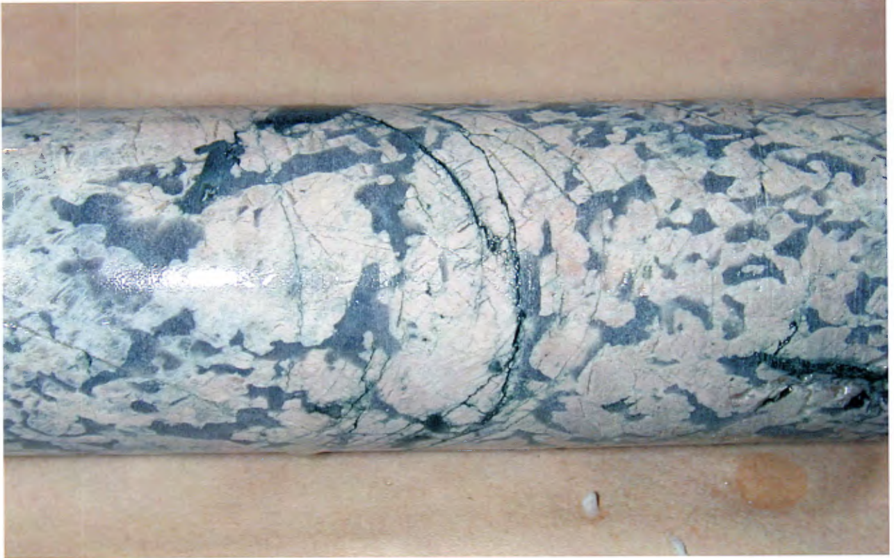
Plate 19 Graphic intergrowths of quartz and feldspar in pegmatite (hole 2004 @ 91 m).
