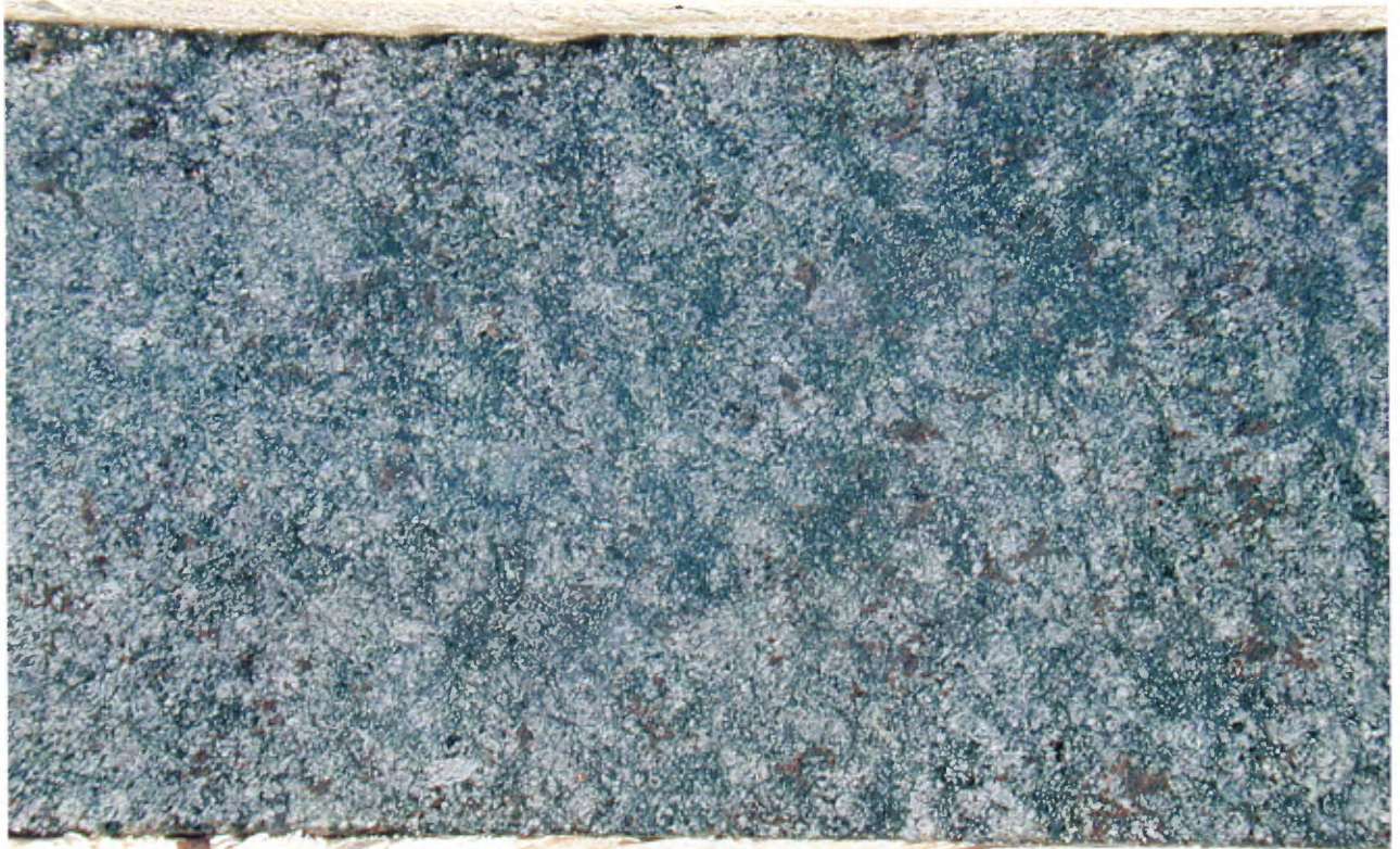
Plate 12 Strongly magnetic, course-grained, dark green, serpentinized peridotite (hole 2004 @ 136 m).
