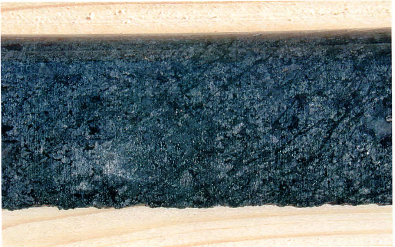
Plate 13 Moderate development of foliation in serpentinized peridotite is apparent on the reverse side of sample in plate 12 (hole 2004 @ 136 m).
