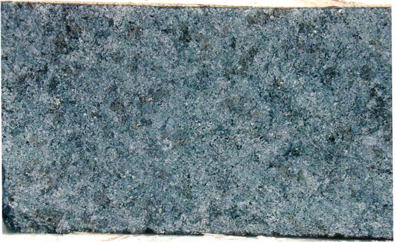
Plate 11 Weakly magnetic, medium to coarse-grained, intergranular, creamy green olivine gabbro (hole 2006 @ 82.5 m).
