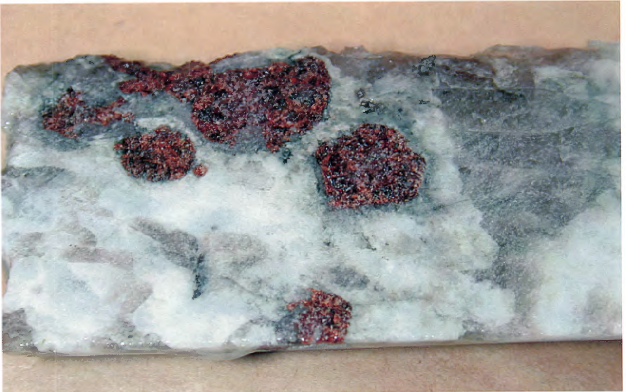
Plate 17 Accessory garnets in graphic pegmatite (hole 151-05 @ 407.5 m).
