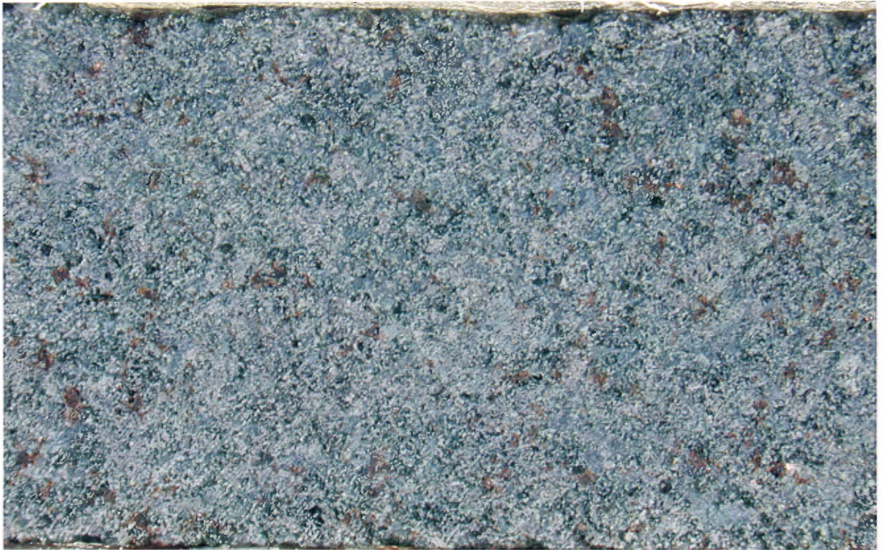
Plate 10 Weakly magnetic, medium to coarse-grained, intergranular, gray-bluish olivine gabbronorite (hole 2006 @ 37.5 m).
