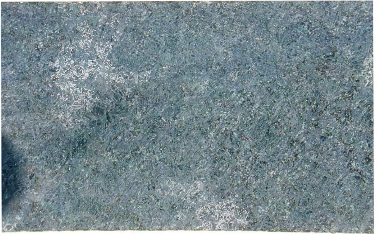
Plate 9 Moderately magnetic, fine to medium-grained, intergranular, gray-green, Ti-rich olivine gabbronorite (hole 2006 @ 177 m).
