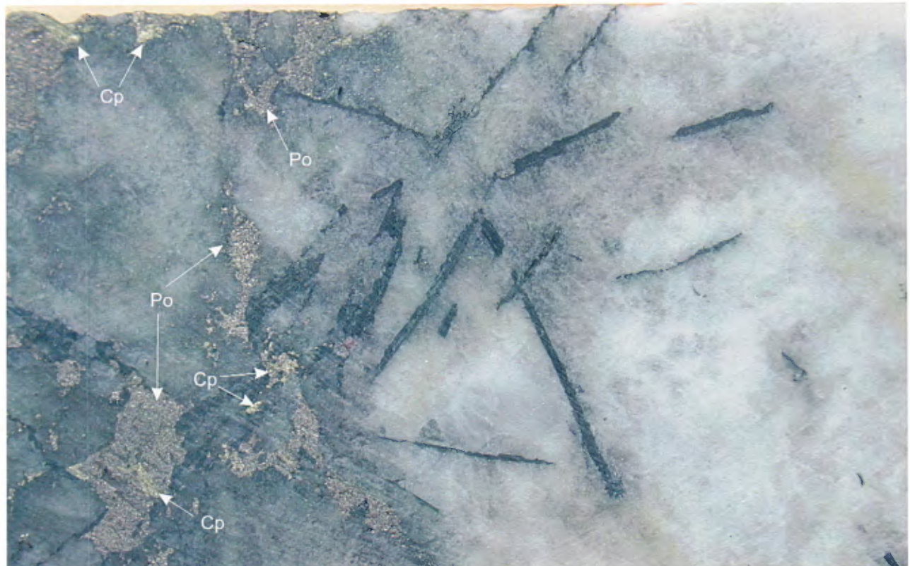
Plate 16 Accessory biotite and hornblende at the margin of a tonalitic pegmatite. Intergranular pyrrhotite (Po) and chalcopyrite (Cp) invading the pegmatite (hole 2002 @ 176 m).
