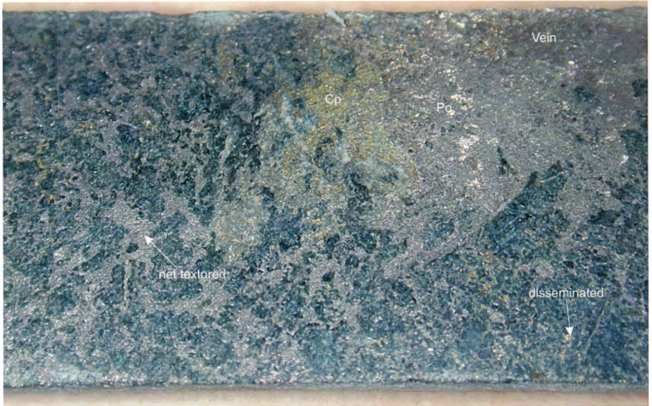
Plate 35 Disseminated and net textured pyrrhotite and chalcopyrite coalesce into a centimetre thick sulphide vein in norite (hole 151-04 @ 201 m). This small-scale feature mimics and clearly illustrates the formation of the large-scale massive sulphide veins.
