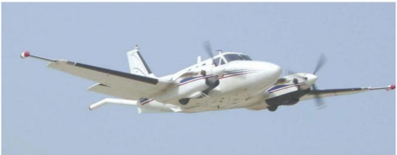
Figure 11. Beechcraft King Air used to conduct the Eldor Property survey in 2007. Magnetic sensors were carried in wing-tip pods and tail-mounted stinger. Spectrometer detectors (33.6 litres) were carried on board. Photo courtesy Tundra Airborne Surveys Ltd.
