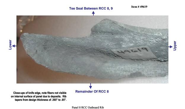
Figure 5-4. Example of rib erosion
