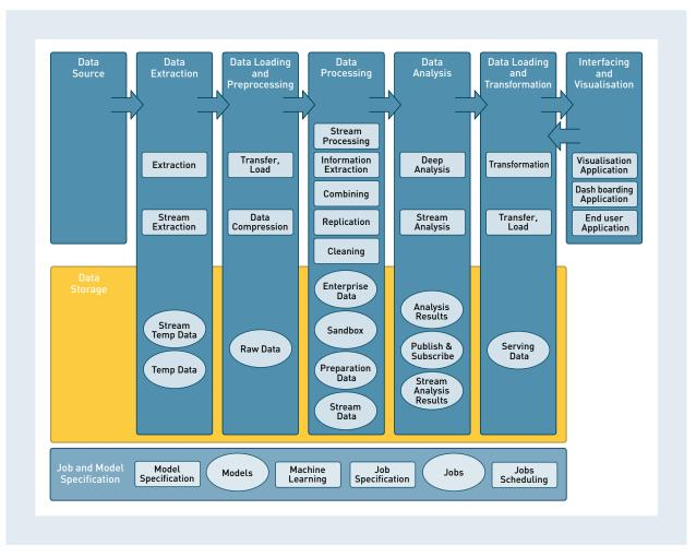
Figure 28 – A technology-independent Big Data Analytics reference architecture [147]
