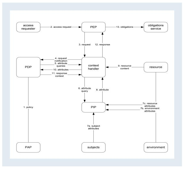
Figure 29 - XACML Dataflow [148]
