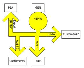
Fig.5. Load flow diagram of a chosen SPP
