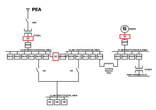
Fig.6. Installation diagram of additional reactors.
