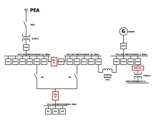
Fig.11. Installation diagram of FCL (I1, I2 and I3).
