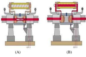
Fig.2. Current limiting devices by ABB [5], [6].
