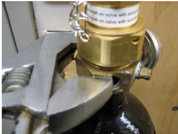
Figure 1. Outlet Fitting (P/N: WK-699205-010) Removed and Wrench Shown on Valve Flats
