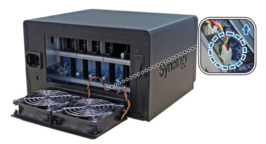
c Remove the 4 screws that secure the malfunctioning fan, and then remove the fan.
