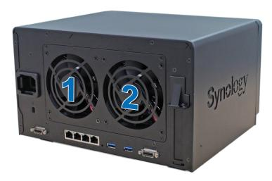
3 Remove the 4 screws that secure the fan panel.
