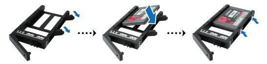
3 Insert the loaded drive tray into the empty drive bay, and press the handle in flush with the front panel to hold the drive tray in place.
