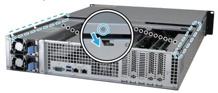
**b** Put back and fasten the screw you removed in step 2-a.
