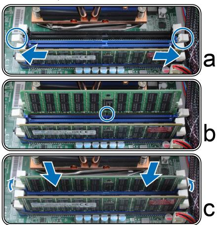
*Note:* Hold the memory module by its edges, and do not touch the gold connectors.
