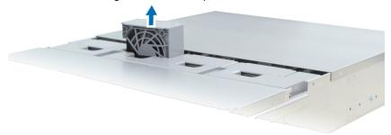
**5** Prepare a new fan, and slide it into the FlashStation. Make sure the fan is aligned properly as illustrated below.
