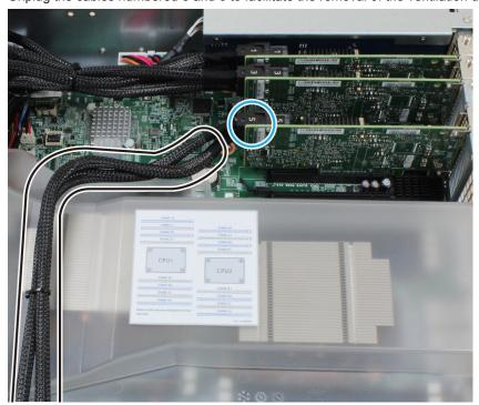
**5** Remove the 3 screws that secure the ventilation duct cover, pull up the ventilation duct cover, and put it aside.
