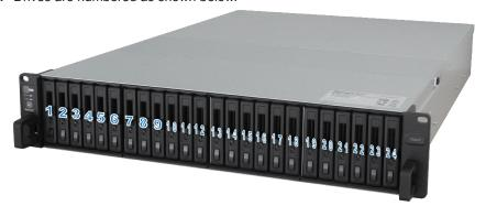
**Note:** If you want to create a RAID volume, we recommend all installed drives be the same size in order to optimize drive capacity usage.
