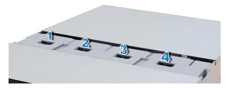
4 Find the malfunctioning fan. Lift up the fan to remove it.
