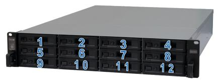
**Note:** We suggest installing drives of the same size to optimize drive capacity usage when creating RAID volumes.
