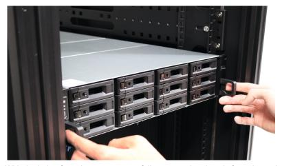
2 With the help of another person, carefully remove the chassis from the rack. Then, slide forwards to remove the inner rail from the chassis.
