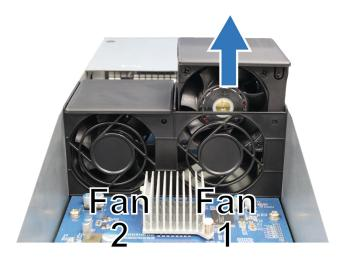
2 Prepare a new fan, align the arrow to point at the back panel as illustrated below, and insert it back into the fan slot.
