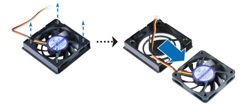
**5** Slide a new fan into the fan case. Tighten the screws to secure the fan in place.
