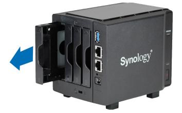
2 Place a drive in the drive tray. Turn the tray over and tighten the screws provided to secure the drive in place, as illustrated below.
