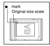
Place the original face down on the document glass. Align the corner of the original with the tip of the arrow mark ( ) on the document glass scale.
