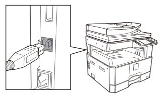
(3) Connect the other end of the cable to the USB connector (A type) on your computer.
