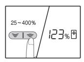
Press the [Copy ratio] keys (\$\subseteq\$, \$\subseteq\$) to adjust the ratio in increments of 1%.
