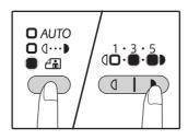
For a darker image, press the [Dark] key ( ). For a lighter image, press the [Light] key ( ). If exposure level 2 or 4 is selected, the two indicators will light simultaneously.
