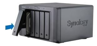
**Note:** Make sure the tray is pushed in all the way. Otherwise, the drive might not be able to function properly.
