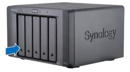
2 Pull the drive tray handle in the direction as indicated below to remove the drive tray.
