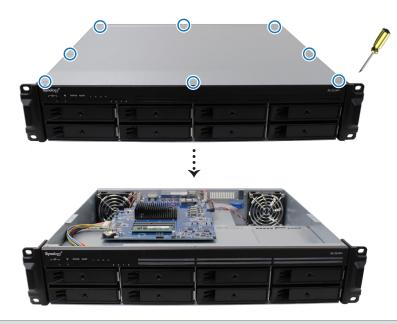
**Note:** When you remove the top cover, sensitive internal components are exposed. Avoid touching anything other than the memory assembly when removing or adding memory.
