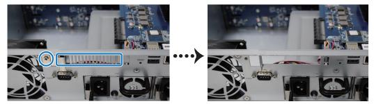
**b** Align the card's connector with the expansion slot and insert the card into the slot.
