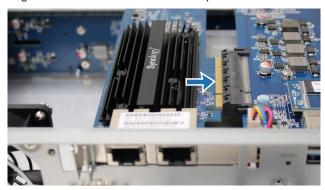
**c** Place back the latch and fasten the screw that you removed in step 2-a to secure the newly inserted card in place.
