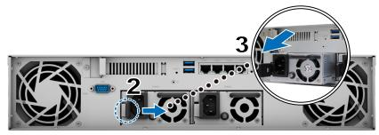
4 Prepare a new PSU. Insert it into the empty slot until you hear a click.
