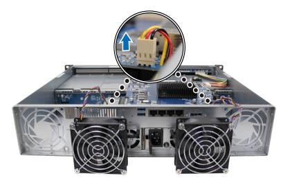
**b** Remove the screws that secure the fan guard from the malfunctioning fan.
