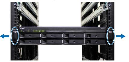
2 With the help of another person, carefully remove the chassis from the rack. Then, slide the inner rail attached to the chassis toward the front panel of the chassis to detach it.
