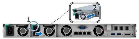
3 Prepare a new power supply, and push it back to the slot unit until you hear a click.
