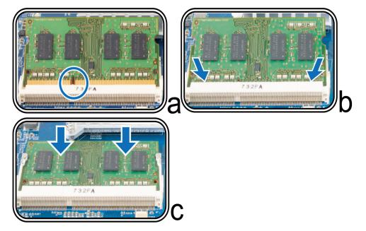
Important: Hold the memory module by its edges, and do not touch the golden connectors.
