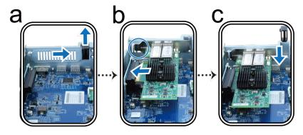
*Note:* Make sure the connector is fully inserted. Otherwise, the network interface card might not be able to function properly.
