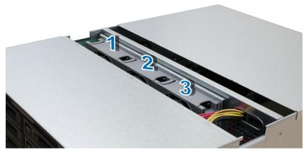
4 Find the malfunctioning fan. Lift the fan upward to remove it.
