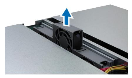
5 Prepare a new fan, and slide it into the RackStation. Make sure the fan is aligned properly as illustrated below.
