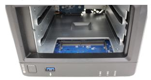
**Note:** When you remove the drive trays, sensitive internal components are exposed. Avoid touching anything other than the memory assembly when removing or adding memory.
