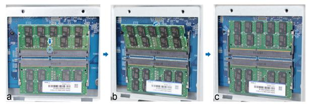
*Important:* Hold the memory module by its edges, and do not touch the golden connectors.
