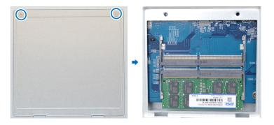
*Important:* When you remove the lid, you expose sensitive internal components. Avoid touching anything other than the memory assembly when you remove or add memory.
