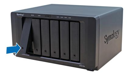
2 Pull the hard drive tray handle in the direction as indicated below to remove the hard drive tray.
