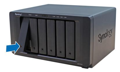
2 Pull the hard drive tray handle in the direction as indicated below to remove the hard drive tray.
