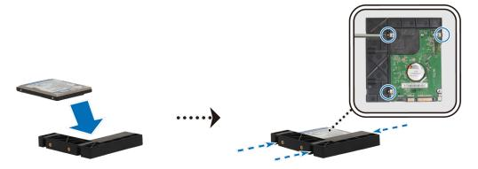
**b** Slide the 2.5" Disk Holder into the hard drive bay, and push it all the way until the drive is firmly connected to the SATA connector. Secure the Disk Holder with the provided screws.
