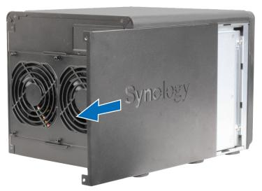
**Note:** When you remove the case, you expose sensitive internal components. Avoid touching anything other than the memory assembly when you remove or add memory.
