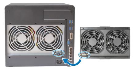
**b** Make sure all six push pins are pulled outwards before the module is attached, and then press the push pins back into place to secure the fan module.
