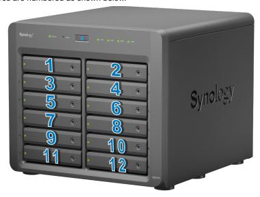
**Note:** If you want to create a RAID volume, we recommended that all installed drives are of the same size to make the best use of drive capacity.
