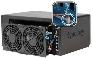
c Remove the 4 screws that secure the malfunctioning fan, and then remove the fan.
