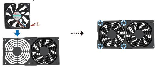
**b** Connect the 2 fan cables to the connectors located near the bottom of the fan socket, and then replace the fan panel.
