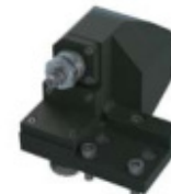
5540-000345 CIT-VDF201-GSI Round Shank Tool Holder M16 Tool Size: Ø19.05mm Single Ended
