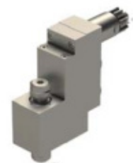
MSE-1007 End Drill/Mill Collet Size: ER11 Output: 1:1 Requires 3 Positions
