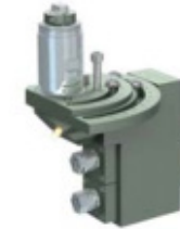
TSU-5540-000220 End Drilling / Milling Main Spindle Collet Size: ER16A Output: 1:1 Adjustable 0-90° Double Ended Holds 4 Tools
