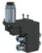
5540-000128 STA-R093-DE2E1611 End Drilling / Milling SR-20J Tool Size: ER11, ER16 Output: 1:1 Double Ended, ER16 front fac- ing, ER11 back facing
