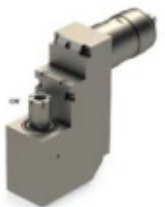
B026-RSE-110M-IK Axial Drilling / Milling Collet Size: ER16 Output: 1:1 Internal Coolant-Thru Machine: B026/32/38
