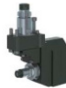
5540-000455 STA-5540-000455 Slitting Saw SR-20R Sub Spindle Tool Size: Ø6mm Output: 1:0.55 Adjustable +/- 1mm, Single Ended, Max Tool Ø50mm
