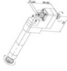
GSE-306-DE011 End Drill/Mill Collet Size: ER11 Output: 1:1 Double Ended
