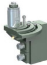
TSU-5540-000220 End Drilling / Milling Main Spindle Collet Size: ER16A Output: 1:1 Adjustable 0-90° Double Ended Holds 4 Tools
