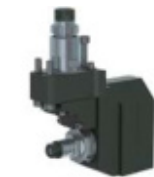
5540-000157 STA-BWSS-5MM Slitting Saw SR-20RIV Sub Spindle Tool Size: Ø5mm Output: 1:0.55 Single Ended, Adjustable +/- 1mm, Max Tool Ø50mm
