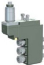
TSU-5540-000254 End Drilling / Milling Main Spindle Collet Size: ER16A, ER11A Output: 1:1 Double-Ended Holds 6 Tools
