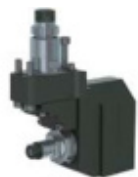
5540-000462 STA-5540-000462 Slitting Saw SR-20RIV Sub Spindle Tool Size: Ø10mm Output: 1:0.55 Single Ended, Adjustable +/- 1mm, Max Tool Ø50mm
