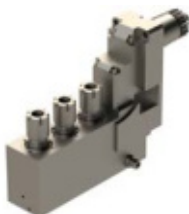
GSE1610-IK End Drill/Mill Collet Size: ER16 Output: 1:1 Internal cooling Max 90 bar, Drill depth 37mm
