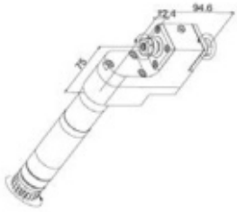
GSE-306-DE312 End Drill/Mill Collet Size: ER11 Output: 1:3 High Speed Double Ended
