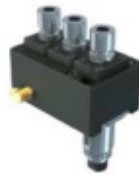
5540-000160 STA-SRBW-3E11 End Drilling / Milling SR-20J Sub Spindle Tool Size: ER11M Output: 1:1 Single Ended
