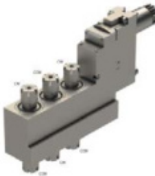
BSA-2010 Angled Drill/Mill Collet Size: ER16 Output: 1:1 Adjustable 0-21° Interferes with adjacent tooling position when used at angle A32 L32
