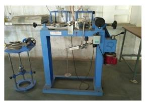
Direct Shear Test Apparatus
