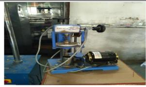
Vane Shear Test
