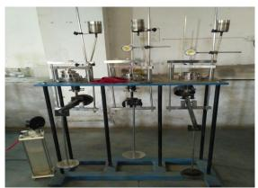
Consolidation Test Apparatus
