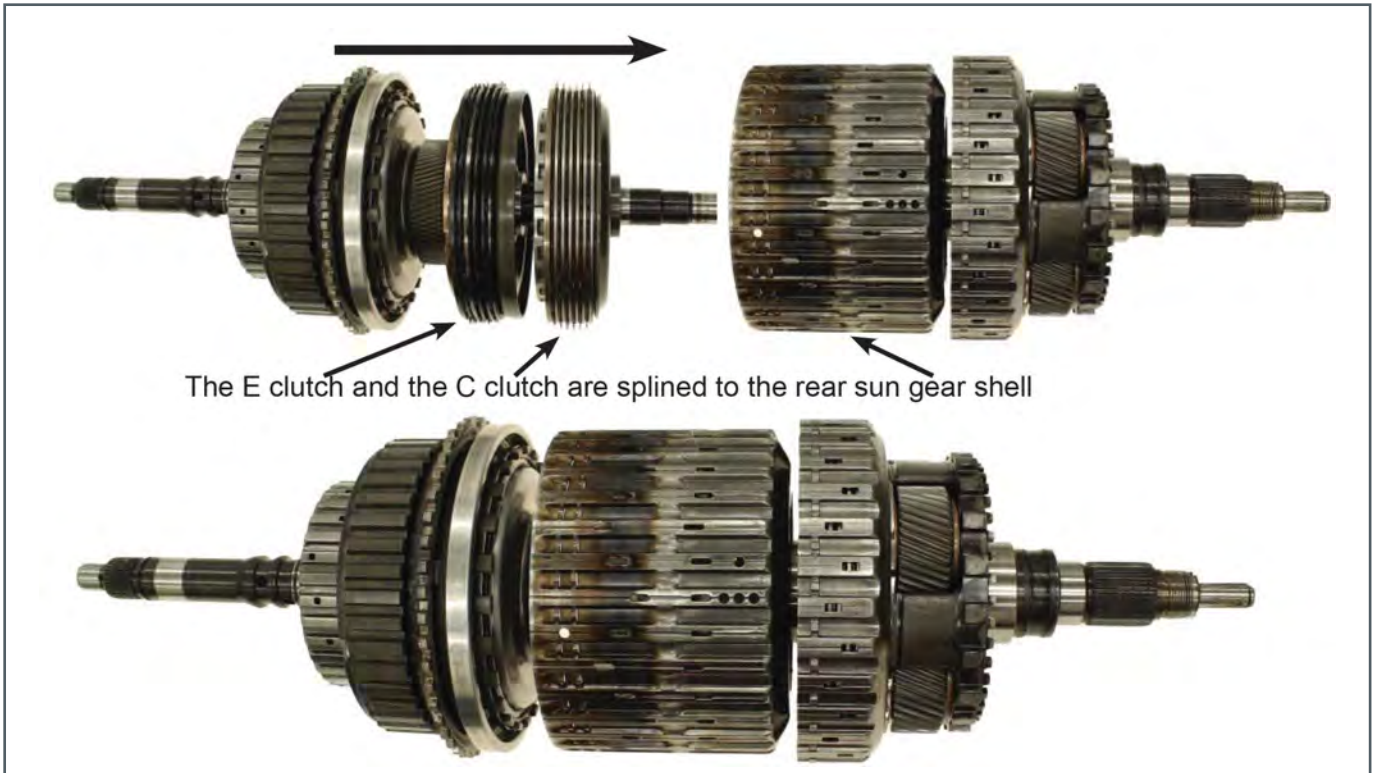
Figure 3: Two clutches splined to the sun gear shell means the sun shell can be driven at two different speeds.
