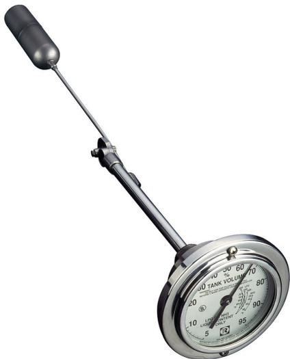
A direct-reading float gauge that is a direct replacement for rotary-type, dip-tube gauges in LP and NH3 storage tanks. Only intended for use in tanks with fixed, liquid-level gauges.
