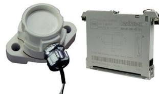
This transmitter is designed to fit Rochester model 6342 and 6360 Magnetel float gauges with 8" dials. The transmitter provides a current output of 4-20 mA proportional to the liquid volume in a horizontal storage tank. Safety barrier provides intrinsic safe outputs.
