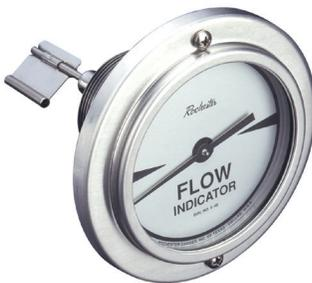
Indicates direction of flow of compatible liquids in pipe lines at working pressures up to 600 psig up to 160°F. The indicator must be installed in pipe line tees. Specify Part Number and "A" Dimension
