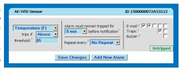
here, you can choose which reading you want to set an alarm threshold on, set the threshold itself, specify whether the alarm is to trip when the monitored temperature goes above or below the desired threshold, and which action(s) are to occur when the threshold is exceeded.
