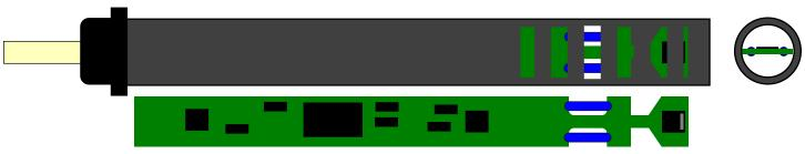
If, on the other hand, the circuit board inside the sensor has a more complex-looking series of cutouts, including two cylindrical components stretched across a pair of U-shaped cutouts, with a single flat square component visible at the spade-shaped tip, it is an RTAFHD3.
