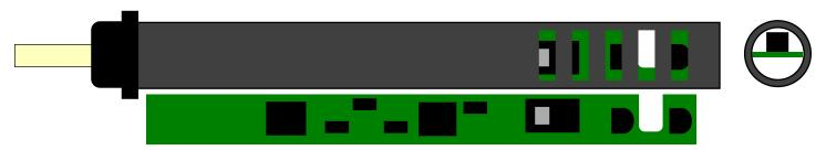
If the sensor is housed inside a grey plastic tube with five or six horizontal slots at one end, examine the circuit board inside the tube through the slots and through the opening at the end. If you see a circuit board with two black, D-shaped components on either side of a single U-shaped cutout, it is an RTAF2 (Temperature/Airflow), RTAFH2 (Temperature/Airflow/Humidity), or RTHD2 (Temperature/Humidity/Dewpoint) device manufactured in 2008 or beyond.
