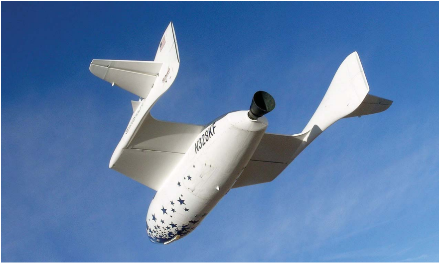
FIGURE 16–3. SpaceShipOne gliding down for landing. This air ship uses a hybrid propulsion system to produce its main thrust. The propellant is N 2 O-HTPB. (Photo by scaled composites. SpaceShipOne is a Paul G. Allen Project © Mojave Aerospace Ventures, LLC.)
