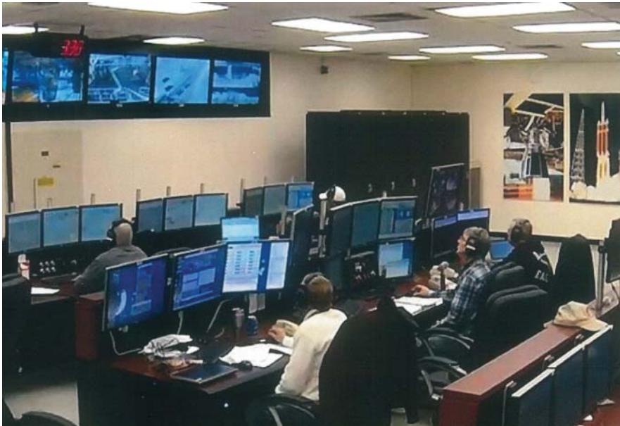
FIGURE 21–3. Photograph of an actual RS-68A acceptance test. The test conductor is in the middle back row; to his right is the engine test article engineer and to his left is the controls and vehicle simulation engineer (the row in front primarily controls facility stations, like the oxygen and hydrogen systems). Up on the top are units monitoring engine firing. Present day testing is nearly all controlled remotely with computers, which also display read-out meters and act as data recorders. Reproduced by courtesy of Aerojet Rocketdyne.
