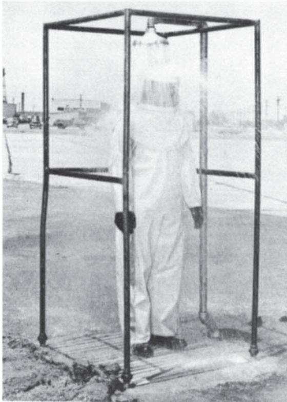
FIGURE 21-4. Plastic safety suit, gloves, boots, and hood used by test personnel in handling hazardous and/or corrosive liquid propellants. The safety shower, which starts automatically when a person steps onto the platform, washes away splashed or spilled propellant. Official U.S. Air Force photograph.
