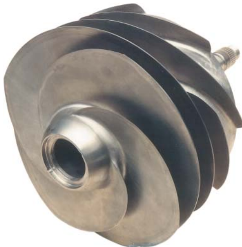
FIGURE 10–9. Fuel pump inducer impeller of the Space Shuttle main engine low-pressure fuel turbopump. It had a diameter about 10 in., a nominal hydrogen flow of 148.6 lbm/sec, a suction pressure of 30 psi, a discharge pressure of 280 psi at 15,765 rpm, an efficiency of 77%, and a suction specific speed of 39,000 when tested with water. Courtesy of Aerojet Rocketdyne.
