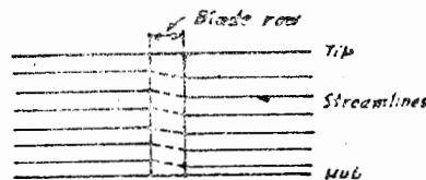
Fig. 7-20. Streamlines under the assumption that all the radial flow takes place in the blade passages.
