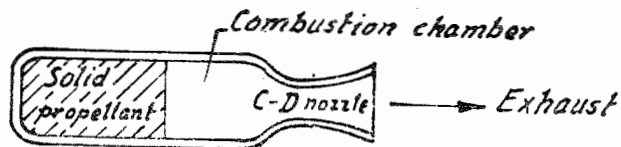
Fig. 9·4 Schematic diagram of solid a propellant rocket
