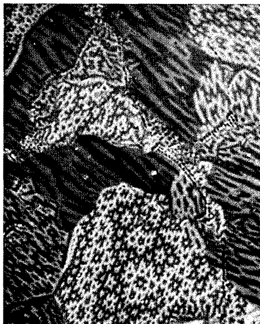
Fig. 519. Magnetic domains in Sm_2Co_{17} . Rosette structure in grain at right is characteristic of easy-axis magnetic symmetry. Characteristic easy-axis domain patterns were seen in Sm_2Co_{17} , Gd_2Co_{17} and R_2(FeCo)_{17} . Domains were not seen in Pr_2Co_{17} , Ce_2Co_{17} , Y_2Co_{17} and Nd_2Co_{17} [72 L 1].
