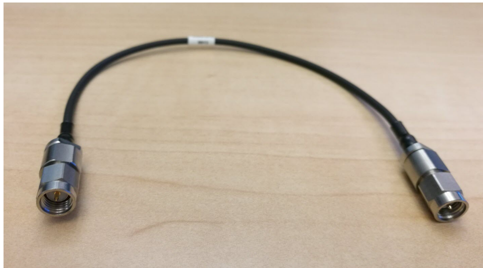
Figure 34: SMA to SMA Cable: Carlisle TM40-0159-00 6"
