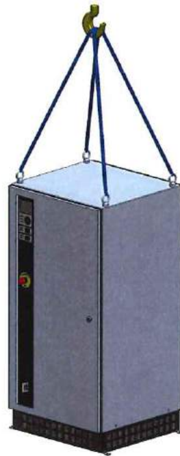
Fig. 4.3.2 Lifting with crane (Place M10 lifting rings at the 4 corners)
