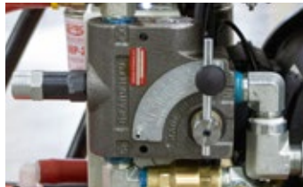
Flow control valve easily adjusts flow rate from 1-8 gallons per minute
