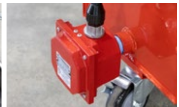
1500 watt heater set at 140°F
