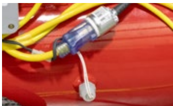
Low fluid heater cutoff float switch
