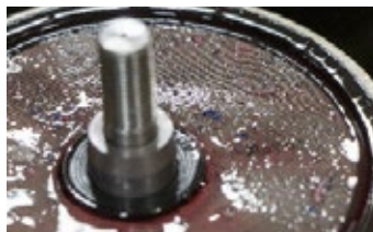
60 micron reusable screen filter verifies cleanliness
