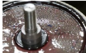
60 micron reusable screen filter verifies cleanliness
