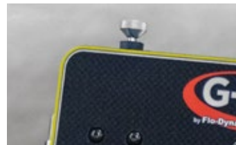
Air purge to additionally agitate during flushing and to clear service lines and cooling system after flushing
