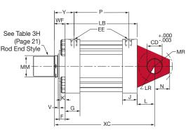
See "CAUTION NOTE" on page 21. **ROD END TRUNNION MOUNT** WF IB EE See Table 3H 00 C (Page 21) 00 Rod End Style D +.000 MŃ 0000 Trunnion pins TL hard chrome plated MODEL HM71 G
