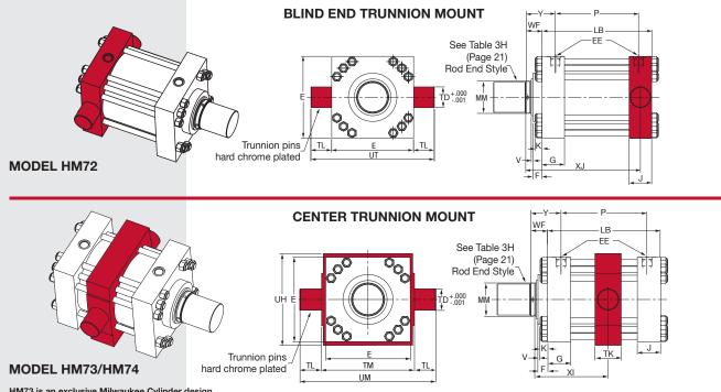
HM73 is an exclusive Milwaukee Cylinder design. HM74 is the Industry "Standard" design. The dimensions given on this table are affected by the piston rod diameter and the stroke.
