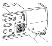
3. Turn the projector upside-down and clean the filter and air intake vents on the base of the projector.
