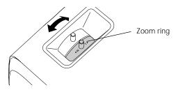
You can also change the image size by moving the projector closer to or farther away from the screen. You can use the E-Zoom buttons on the remote control to zoom in on a portion of the image. See "Zooming Your Image" on page 7 for instructions.
