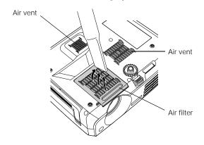
If dirt is difficult to remove or the filter is torn, replace it. The air filter set (part number V13H134A06) contains two filters. Contact your dealer or call Epson at (800) 873-7766 to obtain a new set. In Canada, please call (800) 463-7766 to locate a dealer.
