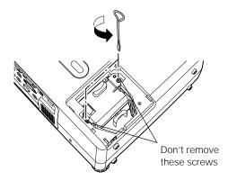
6. Hold the lamp as shown and pull it straight out.
