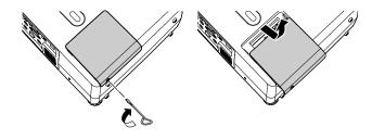
5. Use the screwdriver to loosen the two screws holding the lamp in place. (You can't remove the screws.)
