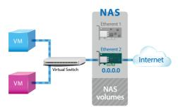
After attaching an Ethernet interface to a Virtual Switch, the IP address of the interface will be changed to 0.0.0.0 so that the VM network traffic will not go throughout the NAS.
