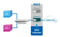
Attaching an Ethernet interface (Port-trunking available) to a Virtual Switch creates a bridged network. The NAS and the Virtual Switch can share the same Ethernet interface without occupation and supports high-speed data transfer via internal routing.
