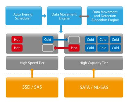
Based on the results of B-tree calculation, the NAS will automatically move data blocks with higher weights to higher tier (e.g. moving data blocks from HDD RAID Group to SSD RAID Group). Here data migration and metadata update will not interfere with normal IO; therefore, transaction-based B-tree update will avoid problems with data integrity.
